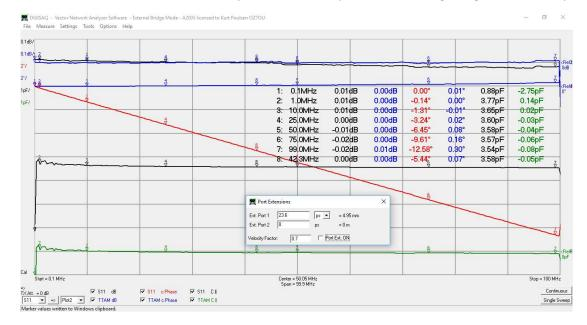
In the Appendix 1 test are made for measuring some SMD resistors from 1 to 10Kohm done before the mathematical custom trace was created, So here a sniff test with the mathematical custom trace for 10hm and 10Kohm. The ImagZ are due to the pin pin lead length of 2x10mm, to which the SMD resistor are soldered. 1 0hm at 1.060hm at 100MHz.
