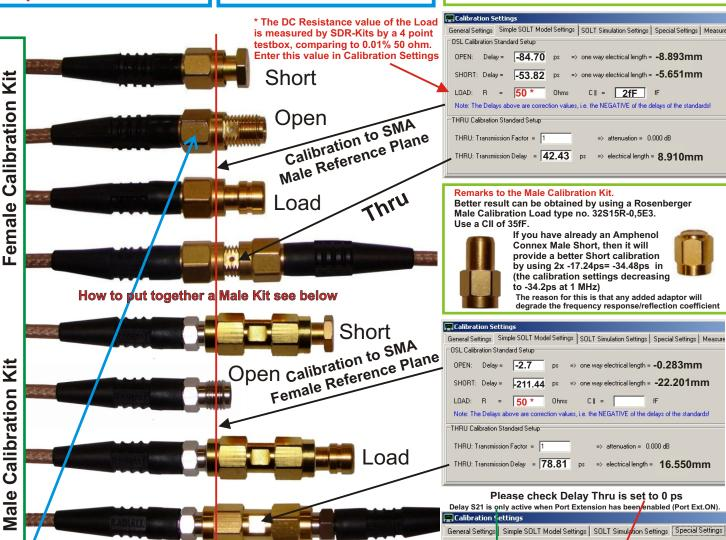
If using an empty Female Thru adaptor (no center conductor no PTFE insert) then the SMA male center conductor is used as the Open standard. Thus the delay used is very small being 2x -5.0ps= -10.0ps.
