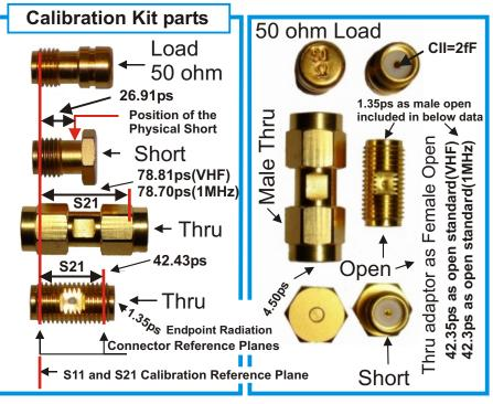
On this sheet you will find the settings required in "Calibration Settings" and "Simple SOLT" for the Reflection (S11/S22) and Transmission (S21/S12)
