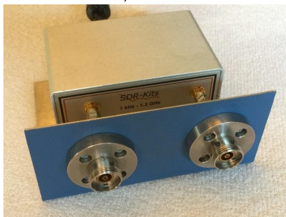
The APC-7 to 3.5mm female flange fitted to the VNWA with two SMA male-male adaptor
