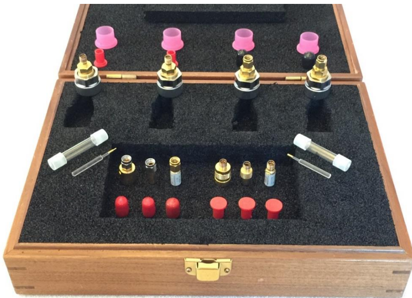
Test equipment for 0.01% precision measurement of load DC resistance
