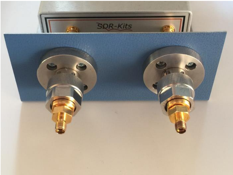
The APC-7 to 3.5mm female adaptors fitted to the VNWA APC-7 frontend to demonstrate the test environment.
