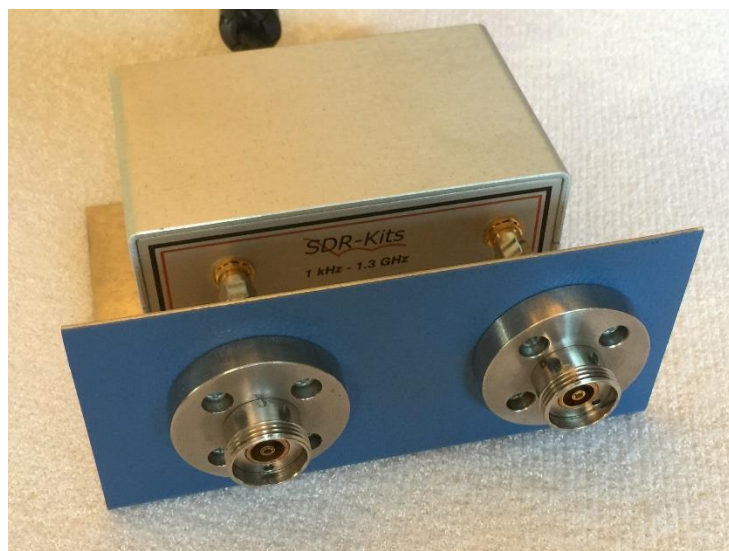
The APC-7 to 3.5mm female flange fitted to the VNWA with a SMA male-male adaptor
