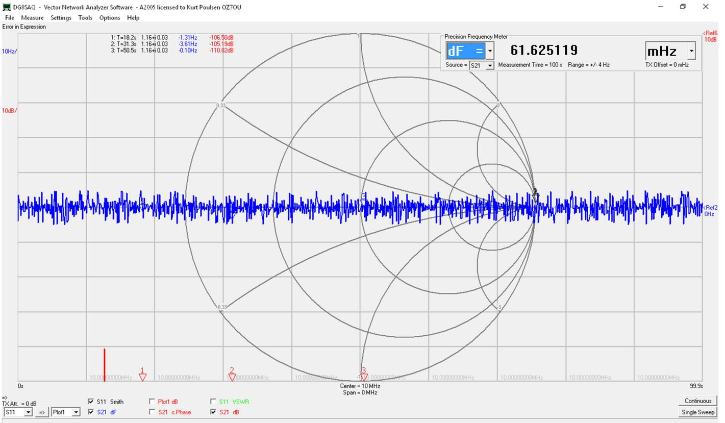
Power interrupted, antenna disconnected and power reapplied. Frequency pretty accurate with noise. Observe dF scale setting 10Hz/div. So a valid GPS signal important for reducing the noise level and if antenna disconnected after a GPS fix the much less noise. Sweep 1000 100ms points.
