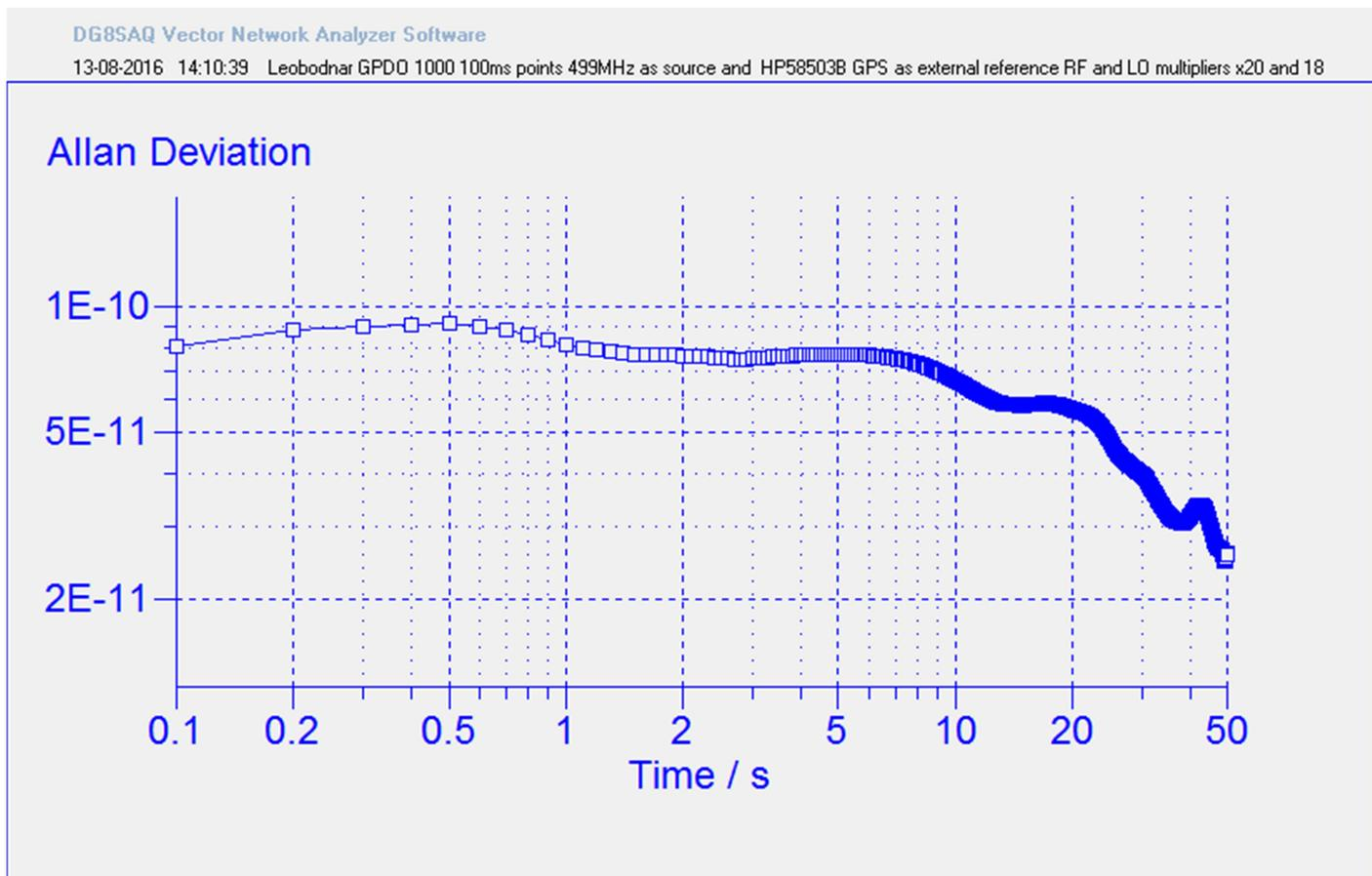
Below a test where the GPS antenna disconnected and shortly after reconnected
