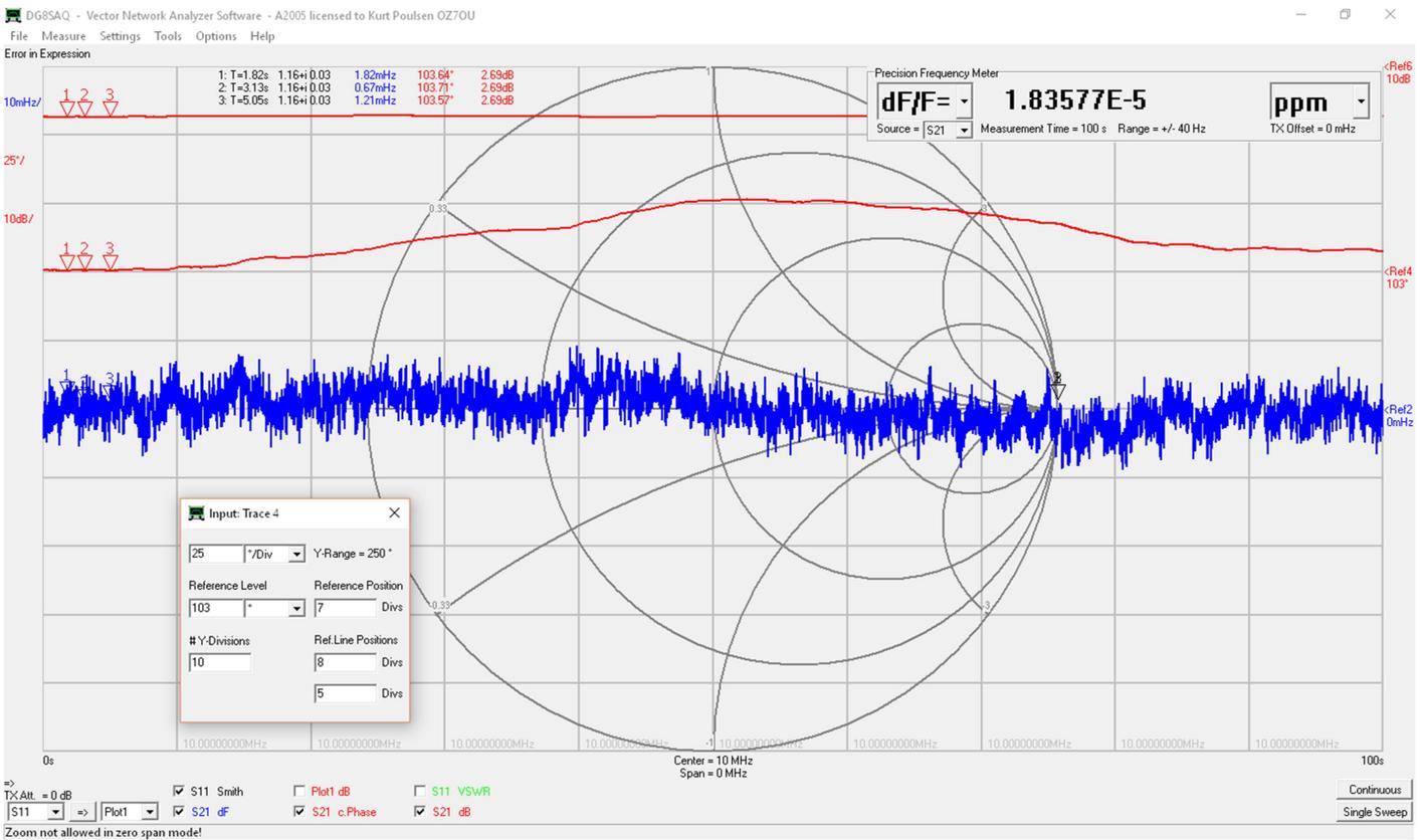
Above Leobodnar GPSDO against HP58503B GPSDO 10000 10ms points demonstrates repeated test not exactly identical
