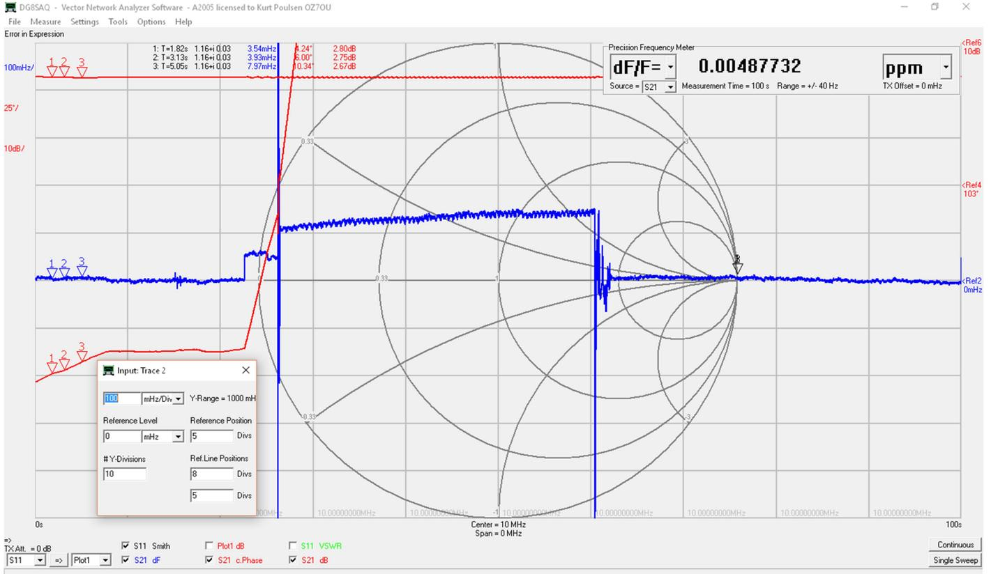
Above Leobodnar GPSDO against HP58503B GPSDO 10000 10ms points GPS Antenna disconnected and reconnected
