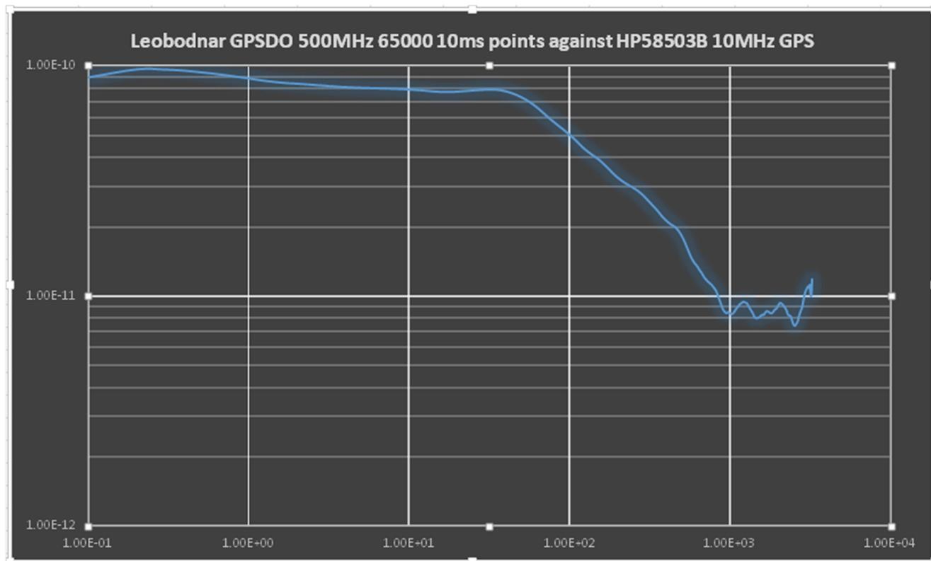
Allan deviation for Leobodnar GPSDO measured for 65000 100mS points at 500MHz against the HP 58503B GPS disciplined 10MHz reference. (Please note an error in the header line not 10ms but 100ms. Below identical plot created by VNWA
