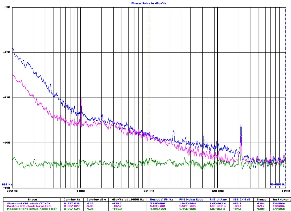
It is now possible to produce phase noise measurement with the VNWA by saving continuous phase \*.dat files and process the in a program called Genplot. A separate document available at the link
