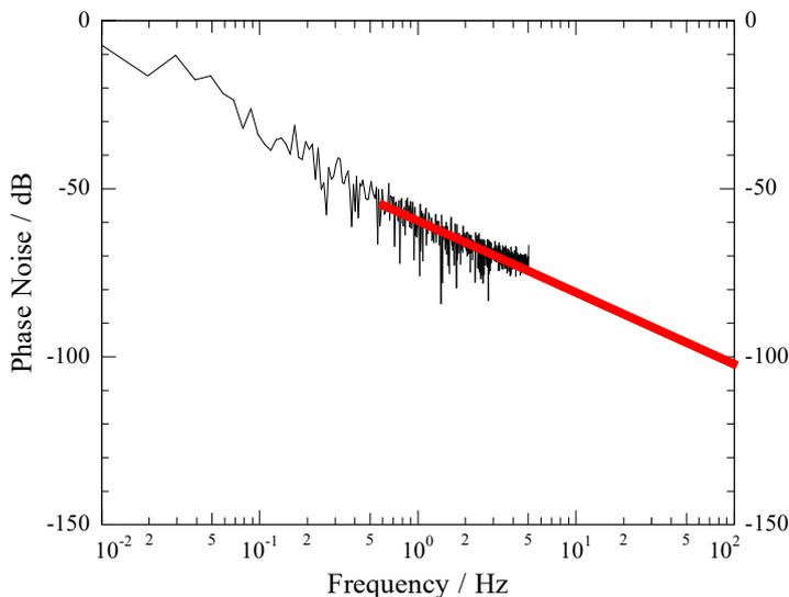
1000 100mS points at 11.9MHz and if a linear curve it will hit about -100dB
