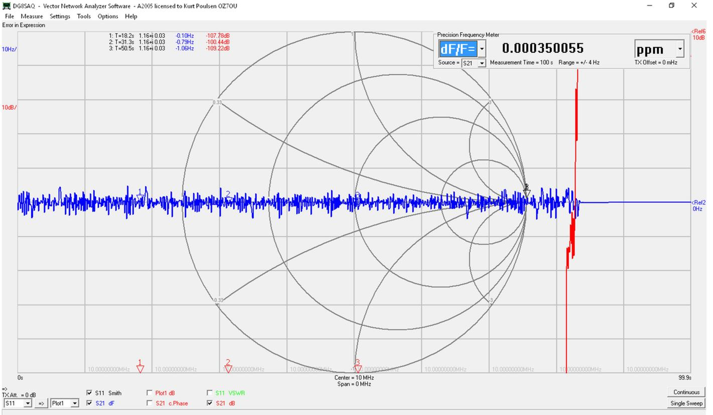
Above when power interrupted, antenna disconnected and power reapplied with antenna connected after 82sec. Sweep 1000 100ms points. Observe the scale setting for dF changed to 10Hz/div
