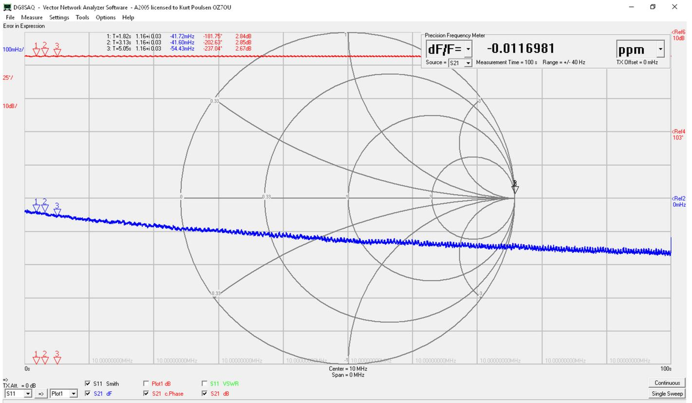
Above shown drift as when GPS antenna disconnected
