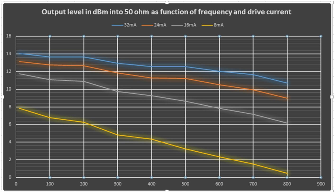
The graphical representation show the effect of the step attenuators 0.1dB resolution and the estimation of + - 0.2dB accuracy seems fair. An averaging/smoothing could be made. The 35 and 50MHz reference signals in the two power meters are to be trusted as correct.
