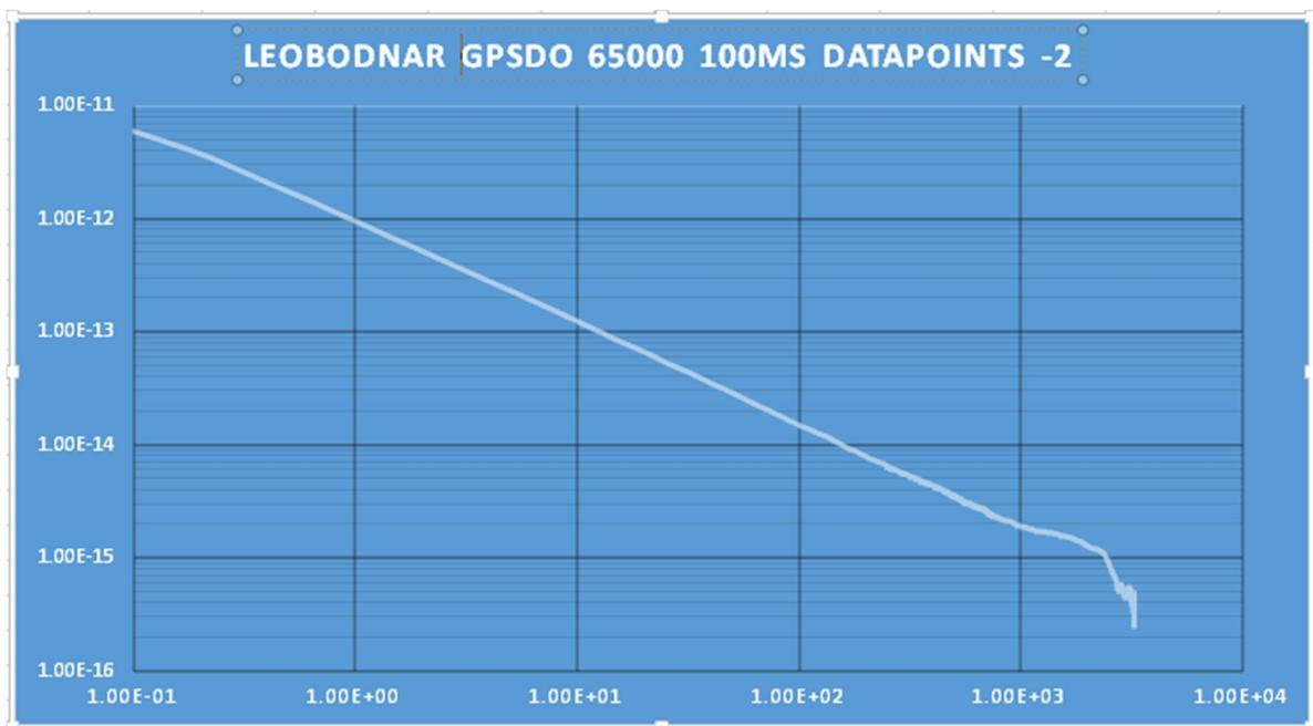
The Allan deviation for above sweep, and it demonstrates excellent risetime for the square wave output, based on experience and many other tests, which will be shown when the HP58503B 10MHz GPS disciplined reference used under same conditions and as the external clock input.
