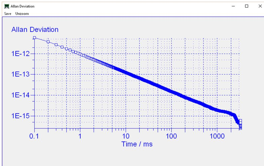
Allan Deviation plot above generated by VNWA for a Leobodnar GPSDO sweep for 65000 100mS points where is it is both signal input and external 10MHz reference. **Please note the Time indicated as ms a small bug now corrected for version 36.6.9.v or later to download from DG8SAQ VNWA Yahoo forum.**
