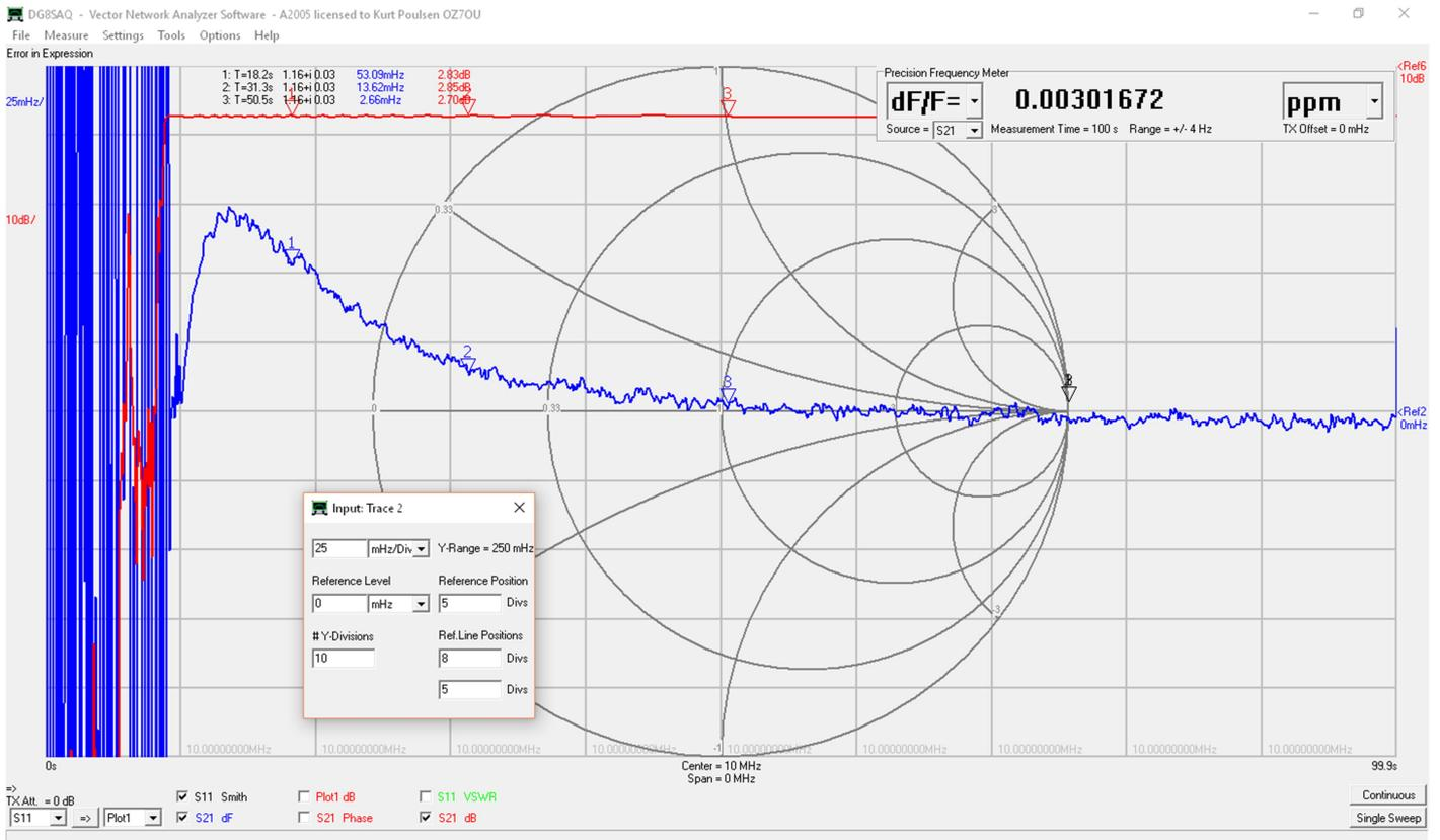
Below demonstrates the result when time per point changed to 10ms for 65000 points which is maximum for a single VNWA sweep. However it is possible to autosave multiple sweeps.
