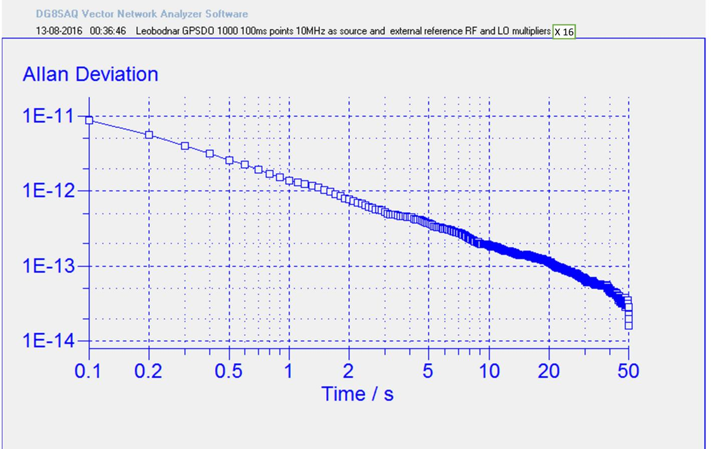
The Allan deviation is almost identical to the sweep with 65000 100mS points so for systems limitation test no need for such many points. The same plot generated quickly by the VNWA software so to speak on the fly.
