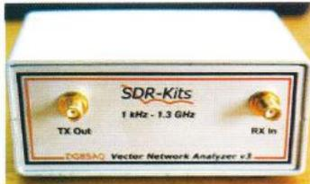
PHOTO 1: The front panel of the VNWA3 with
